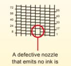
A defective nozzle that emits no ink is substituted with an alternate nozzle.
